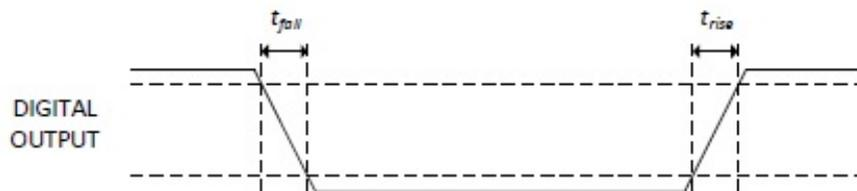
Figure 2: Digital IO Characteristics
