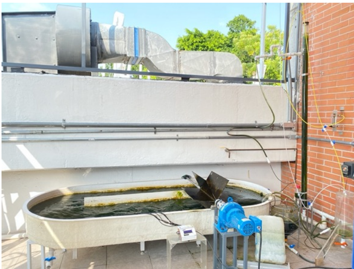
Fig. 40. Photosynthetic biogas upgrading system under environmental conditions at the Institute of Renewable Energies, Temixco, Mexico.
