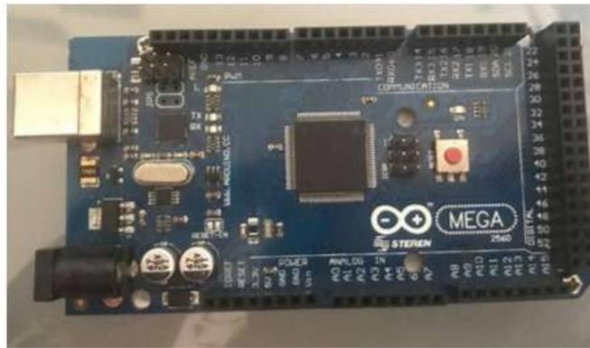
Figura 10: Tarjeta Arduino Mega 2560.
