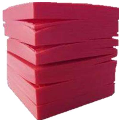
Fig. 50 Cracking. Fuente: <https://www.smallcarsgarage.com/impresoras-3d-fdm/>
