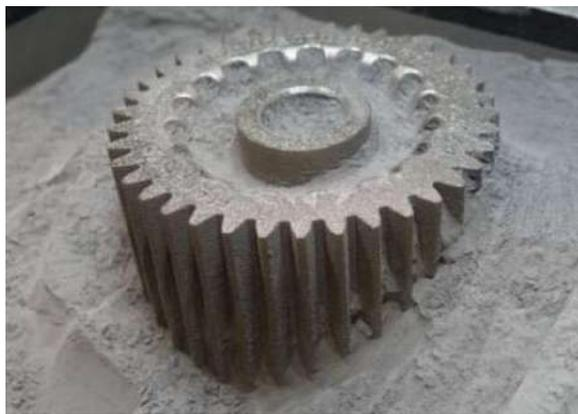
Fig. 18 Sinterizado Láser. Fuente: <https://tu3dprintlab.club/wp-content/uploads/2021/02/powder-3d-printing-900x400.jpg>
