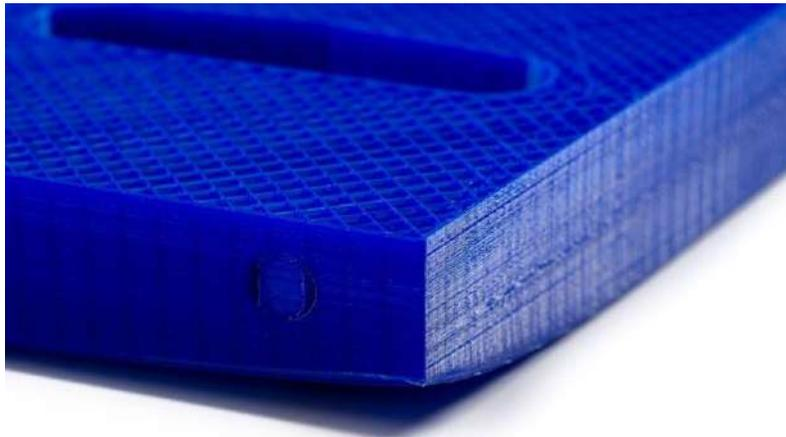
Fig. 49 Warping. Fuente: <https://all3dp.com/2/how-to-prevent-abs-from-warping-on-a-heated-bed/>
