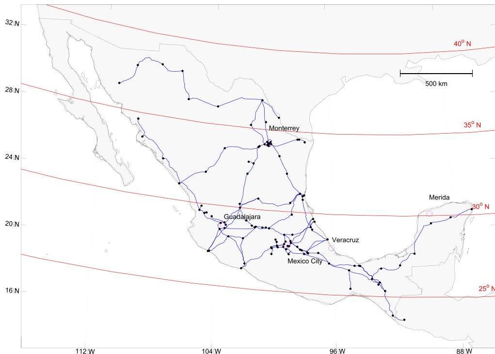
Figure 1. Map showing the Mexican 400-kV power grid, black dots represents substations. Important urban areas are encircled in violet. The red lines represent geomagnetic latitude. Mexico is located at low geomagnetic latitudes and has long power lines close to the shorelines of the Pacific Ocean and the Gulf of Mexico.
