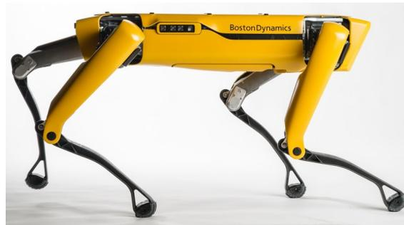
Figura 2.4. Robot spot-mini, Boston Dynamics [5]
