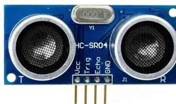
Figura 4.11. Sensor ultrasonico HC-SR04, Hardware Libre [16]
