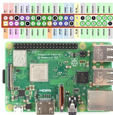
Figura 23. Fuente Raspberry pi spy, diagrama de un mapeo de pines Raspberry Pi, https://www.raspberrypi-spy.co.uk/2012/06/simple-guide-to-the-rpi-gpio-header-and-pins/
