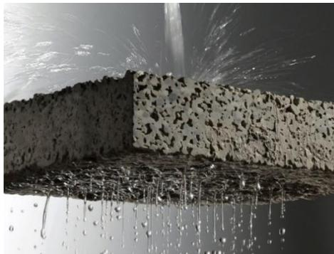
Figura 5. Concreto permeable. (Unknown, 2016)
