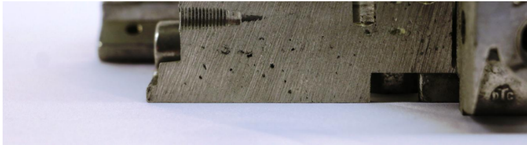
Figura 1.6 Porosidad por gas. International Research Journal of Engineering and Technology (IRJET), 2020.
