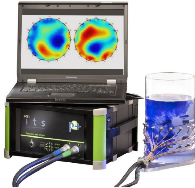
Figure 1.9. ERT system and its comprising units manufactured by ITS ( Sharifi and Young (2013) ).
