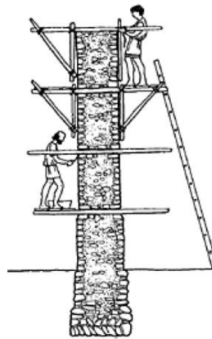
183 Socketed Scaffolding with transverse putlogs.
