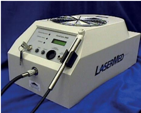
Figura 6. Laser de ion de argón. ( https://www.researchgate.net/figure/Argon-ion-dental-light-curing-laser_fig26_319309779 )
