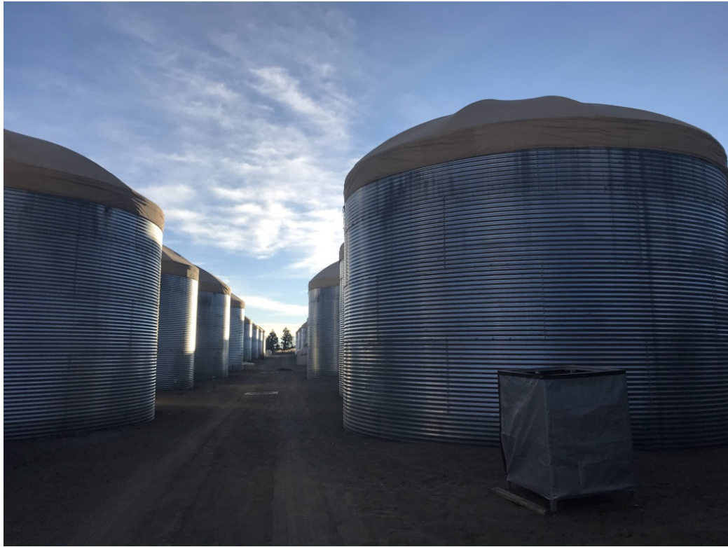
Figure 3.5: One of the two HAWC’s Eye IACTs inside the grey shield, located beside a WCD of the HAWC array.
