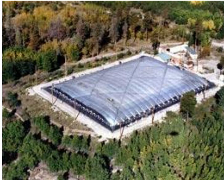
Figure 2.6: The MILAGRO (Multiple Institution Los Alamos Gamma Ray Observatory) consists of a man-made pond lined on the bottom, covered on top, and filled with water. The MILAGRO detector is located in the Jemez Mountains near Los Alamos, New Mexico at an elevation of 2,650 m [MILAGRO, 2021].
