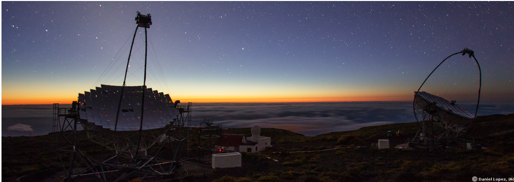
Figure 2.5: MAGIC (Major Atmospheric Gamma Imaging Cherenkov) is a system of two 17 m diameter IACTs. The MAGIC telescopes are located at a height of 2200 m a.s.l. on the Roque de Los Muchachos European Northern Observatory on the Canary Island of La Palma. [MAGIC, 2021]
