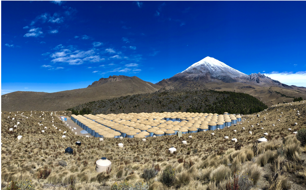
Figure 3.1: The HAWC Observatory. At the center of the array are located the 300 WCD, and in the surroundings are distributed 345 outriggers. In the background, the volcano “Pico de Orizaba” is another active volcano. [HAWC, 2021b]
