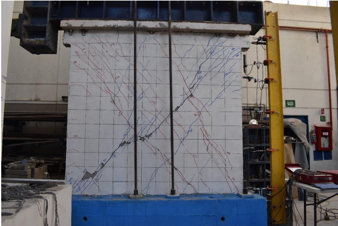
Figura 152. M-7R a \delta = 0.005 . Grieta pico: 3.0 mm, grieta residual: 1.0 mm.
