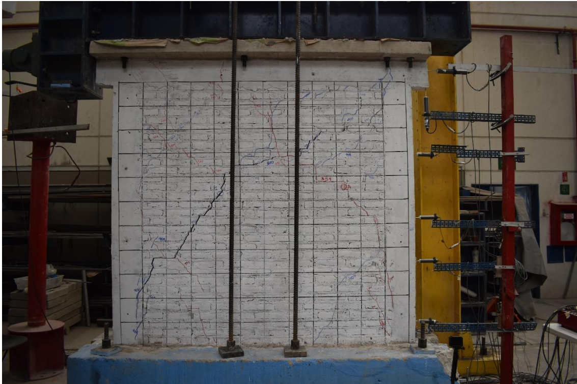
Figura 140. M-5 a \delta = 0.005 . Grieta pico: 7.0 mm, grieta residual: 2.5 mm.
