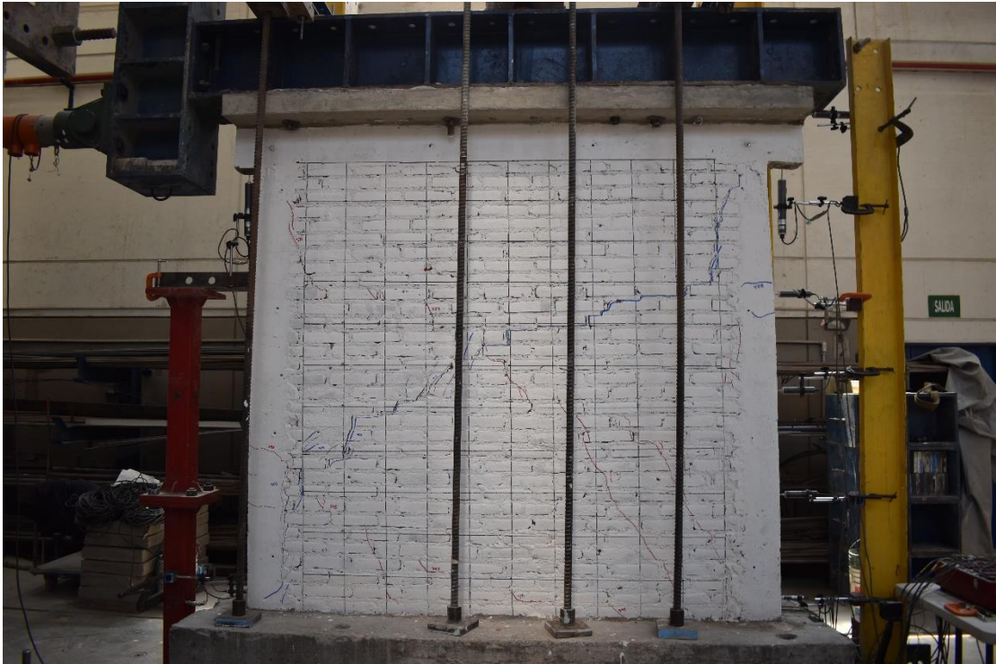
Figura 176. M-13 a \delta = 0.005 . Grieta pico: 5.0 mm, grieta residual: 3.0 mm.
