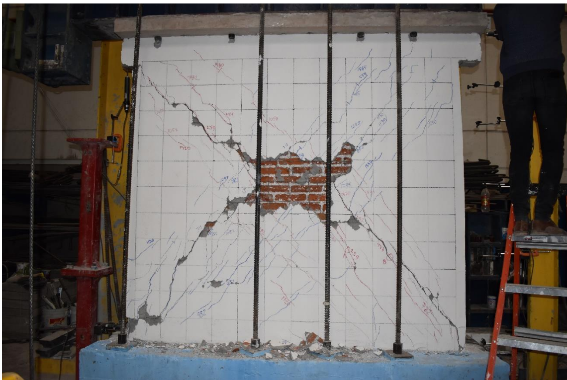
Figura 179. M-13R a \delta = 0.010 . Grieta pico: 5.0 mm, grieta residual: 2.5 mm.
