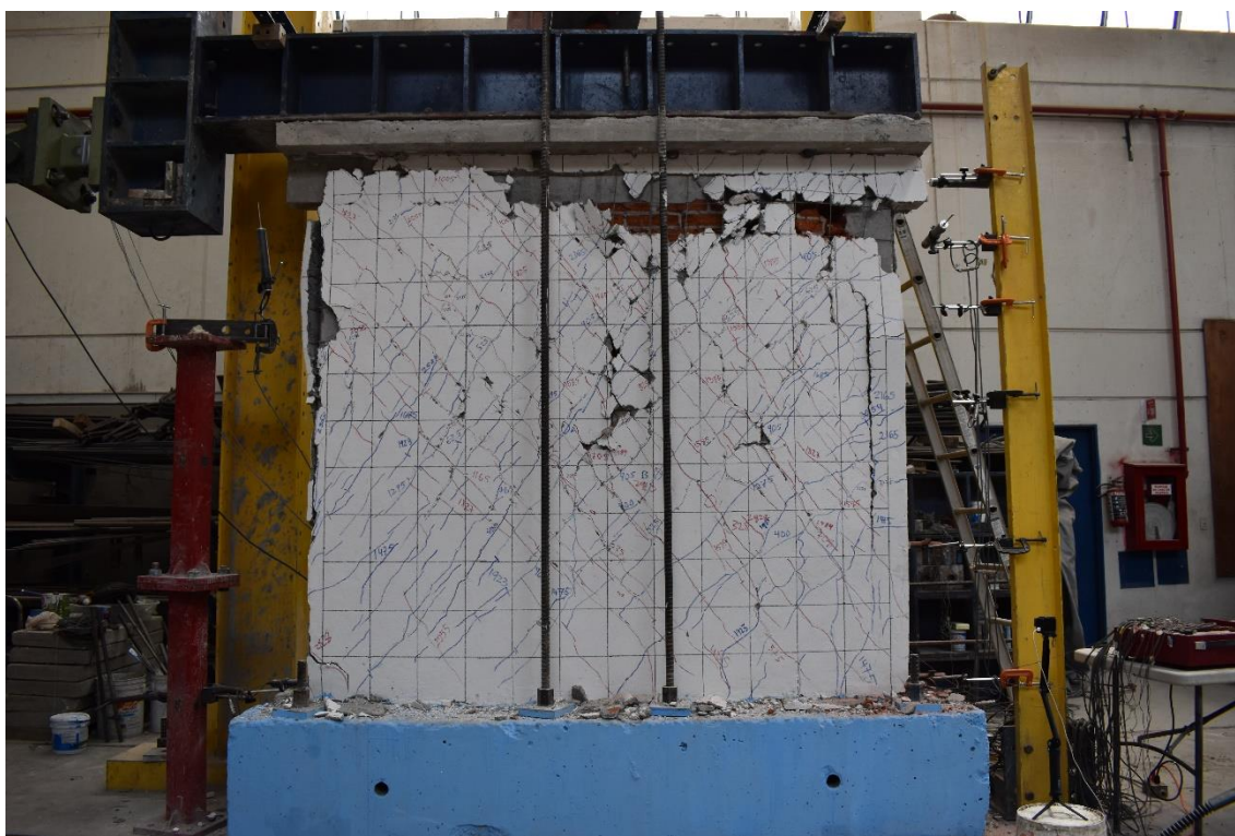
Figura 169. M-11R a \delta = 0.010 . Grieta pico: 2.5 mm, grieta residual: 0.6 mm.
