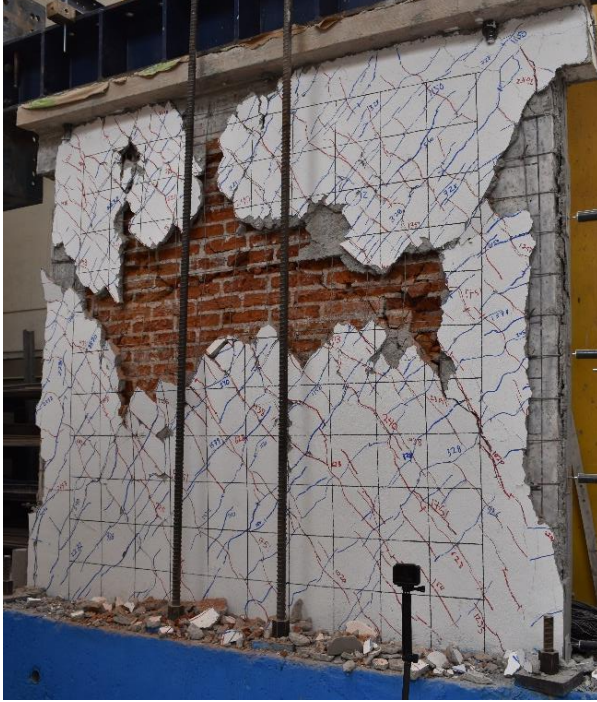
Figura 148. M-6R a \delta = 0.010 . Grieta pico: 2.0 mm, grieta residual: 1.5 mm.
