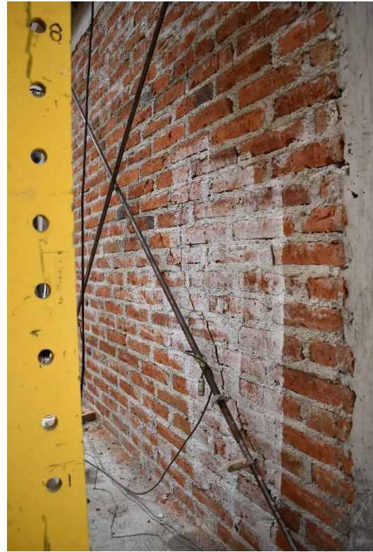
Figura 150. M-7 a \delta = 0.005 . Grieta pico: 9.0 mm, grieta residual: 5.0 mm.
