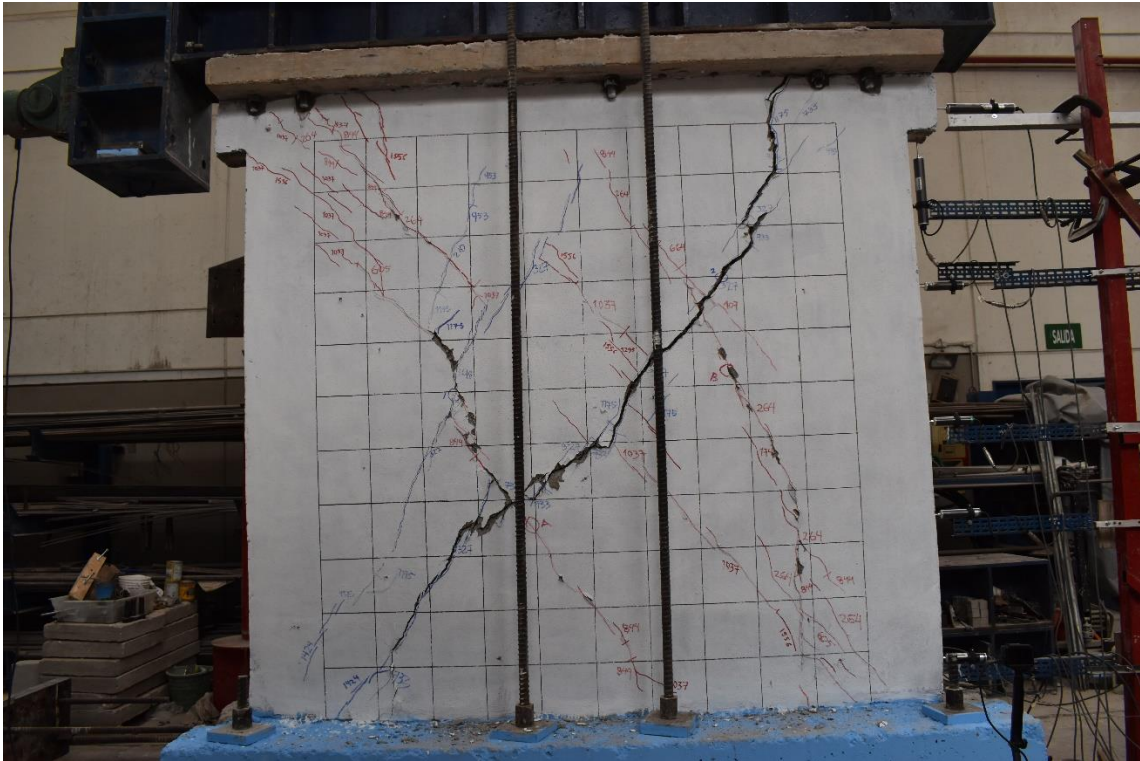
Figura 142. M-5R a \delta = 0.005 . Grieta pico: 2.0 mm, grieta residual: 1.5 mm.
