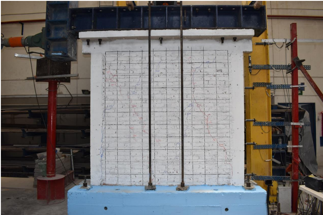
Figura 149. M-7 a \delta = 0.002 . Grieta pico: 2.0 mm, grieta residual: 0.8 mm.
