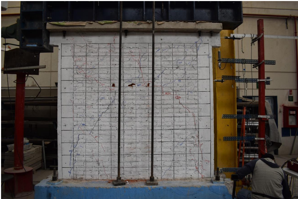
Figura 145. M-6 a \delta = 0.005 . Grieta pico: 10.0 mm, grieta residual: 5.0 mm.
