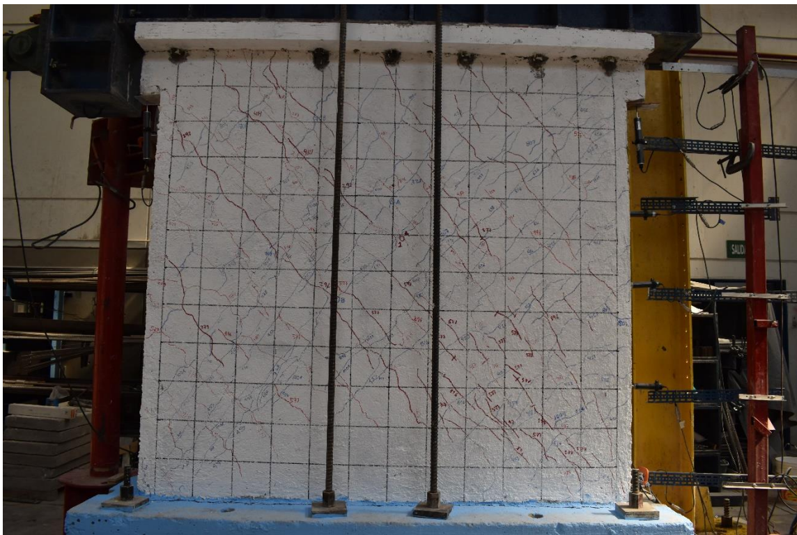
Figura 131. M-2R a \delta = 0.005 . Grieta pico: 1.25 mm, grieta residual: 0.25 mm.
