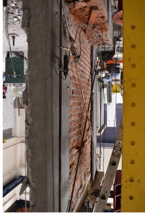
Figura 148. M-6R a \delta = 0.010 . Grieta pico: 2.0 mm, grieta residual: 1.5 mm.
