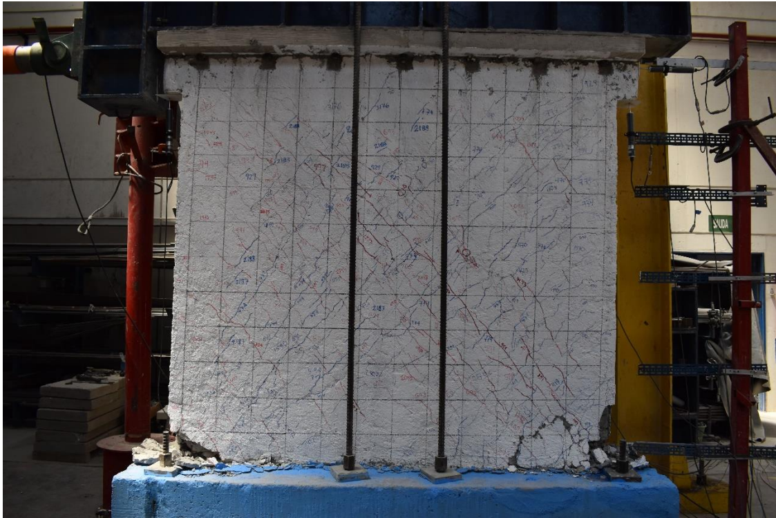
Figura 138. M-4R a \delta = 0.01 . Grieta pico: 1.5 mm, grieta residual: 0.5 mm.
