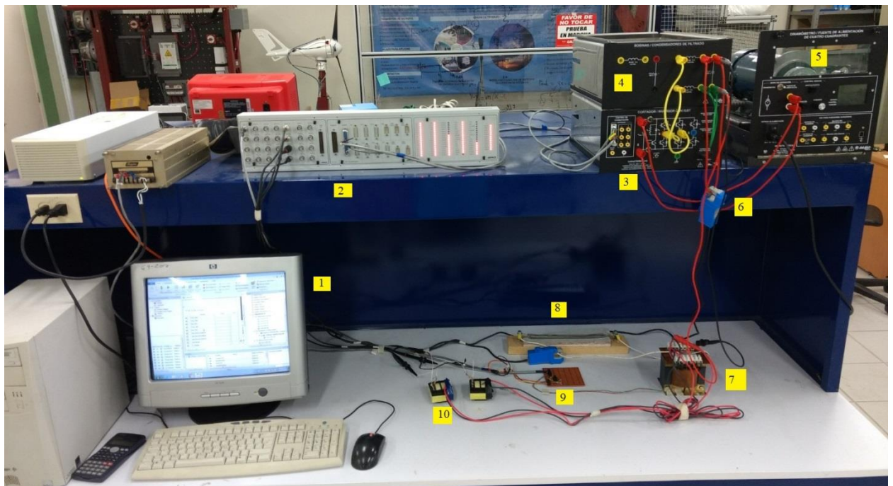
Figure 5.3: Experimental setup; 1) PC 2) dSPACE 3) Inverter 4) filter 5) DC voltage source 0 to 200 V 6) current sensor 7) 200 VA transformer 8) Resistive load 9) Temperature sensor 10) Voltage sensors.
