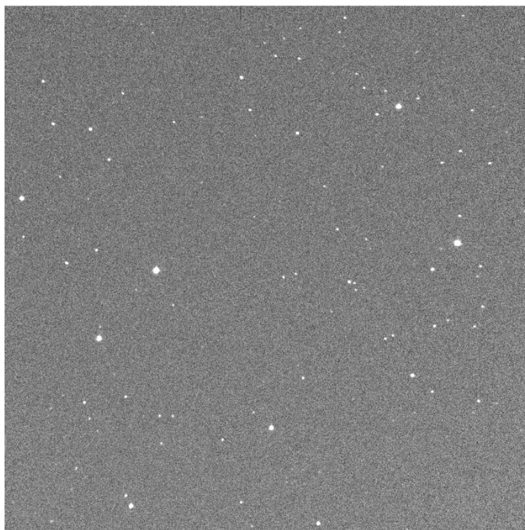
Figure 4.7: Science image that has been calibrated for bias level noise, dark current noise and pixel-to-pixel variation using flat-field images by the CALIBRA program. Once all the science images have been properly reduced we can proceed to the next step of the work done to obtain the transit light curves of a planet. The image shown here is the exact same one that we see in Figure 4.1 from the WASP-69 observation after the calibration was performed.
