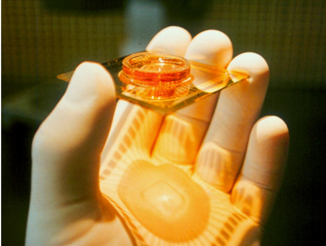
Figura 2. *Multi-electrode array* (MEA). Tomada de Steve M. Potter Lab, “Multielectrode Arrays For Stimulating And Recording Mammalian Neurons”, página web del Georgia Institute of Technology, <https://potterlab.gatech.edu/labs/potter/meas/>, recuperada el 10/07/2021.
