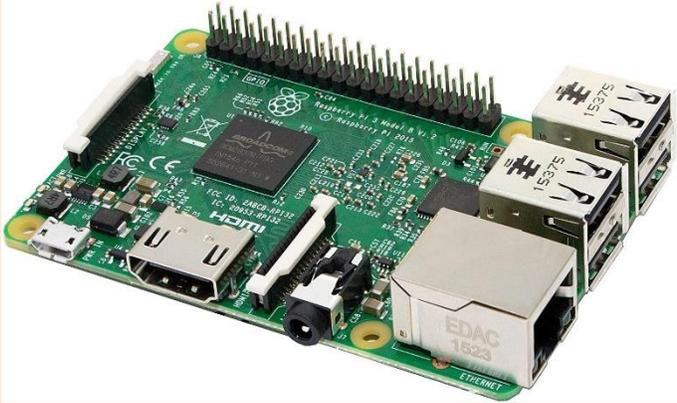
A photograph of a Raspberry Pi 3B single-board computer. The board is green and populated with various components including a central processor chip, a USB Type-C port, an HDMI port, a 40-pin GPIO header, a USB Type-A port, an Ethernet port, and a Micro SD card slot. The board is shown from a top-down perspective. |
