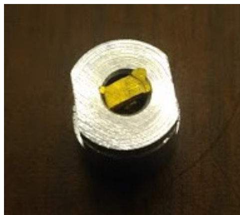
Figure 4.12: Aluminium base cathode with a solid and rectangular gold sample.
