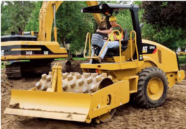
Figura 20. Pata de cabra Caterpillar CS/CP44. (Caterpillar, 2009).
