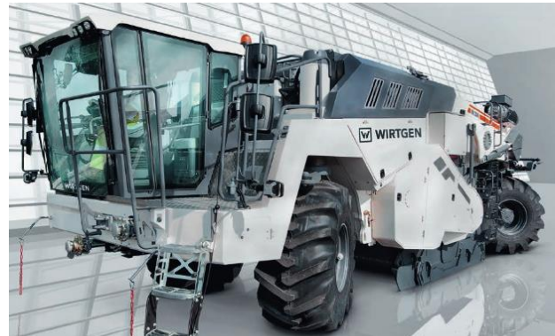
Figura 23. WR XLi Soil Stabilizer Wirtgen. (Wirtgen Group, 2020)
