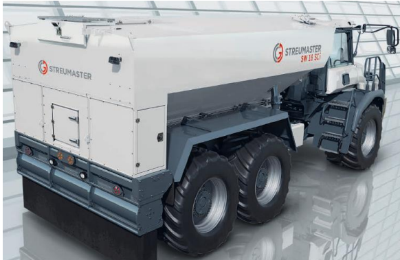
Figura 22. Spreader SW 18 Sci, marca Streumaster. (Wirtgen Group, 2019).
