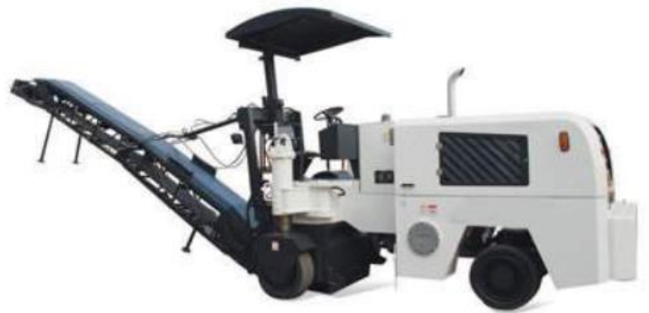
Figura 13. Fresadora LXL1000A (Basso, s/f).
