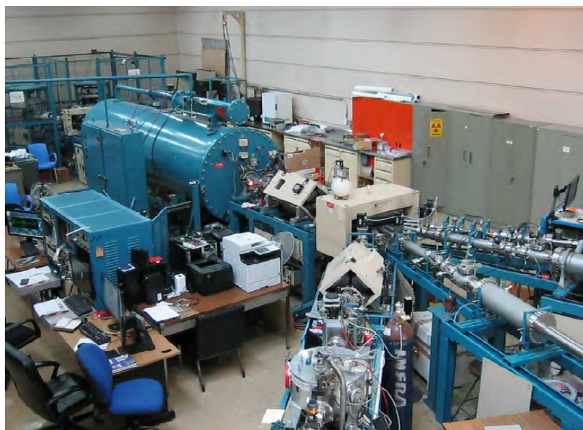
Figure 4.8: An overview image of the 3 MV Pelletron accelerator. The ion sources are located on the top left corner, followed by the main tank on the middle and on the far right the experimental research lines.
