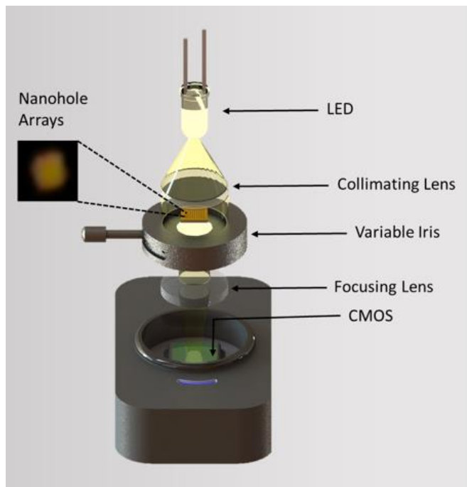
Figure 2.1 Schematic of the SPR imaging experimental setup, displaying the experimental configuration for measuring light transmission through nine arrays of sub-wavelength holes. Magnified image shows the visualised image of nanohole arrays using white LED.
