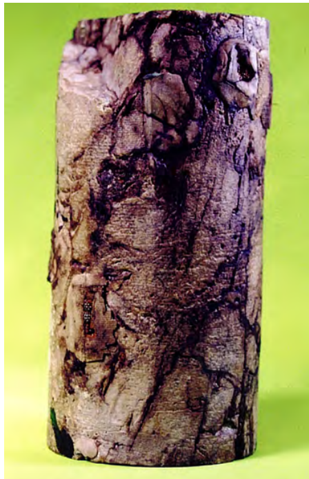
Fig. 2.15: Rock type VI, fractured rock with high fracturing with natural saturation of native residual oil in fractures and matrix.
