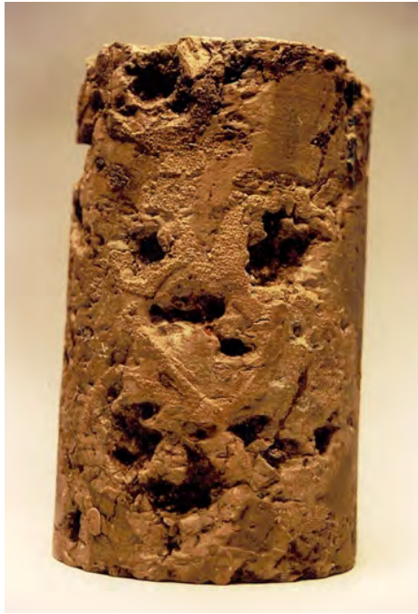
Fig. 2.18: Rock type VII, with representative vuggy- fractures-matrix system.
