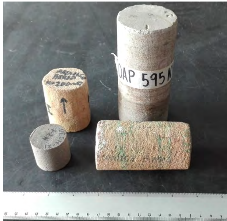
Fig. 1.4: Conventional core plugs used in the petroleum industry.
