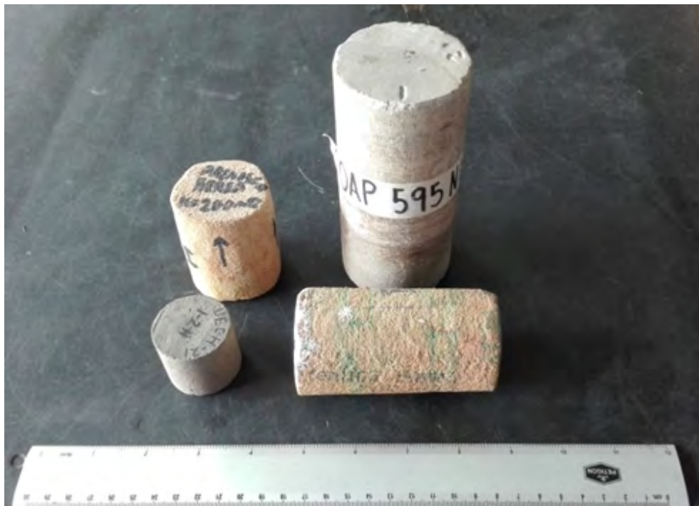
Fig. 2.1: Conventional rock samples used in the oil and gas industry, with a 12 in ruler reference.
