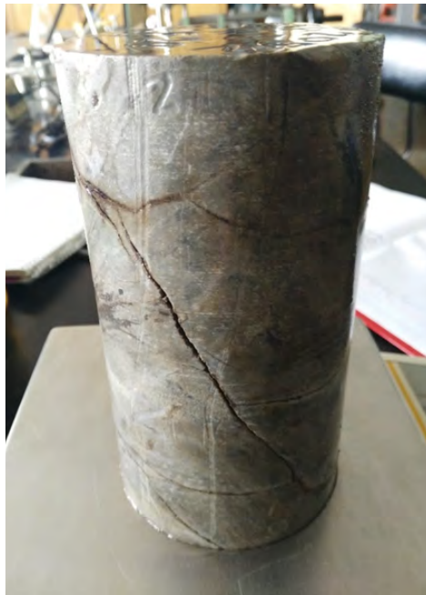
Fig. 2.12: Rock type VI, fractured rock with high porosity and permeability matrix.
