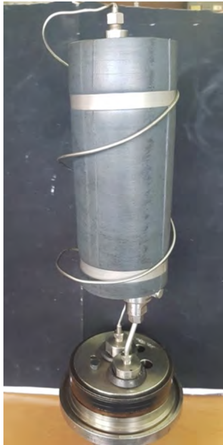
Fig. 4.11: Assembly for core mounting in the high-pressure vessel.
