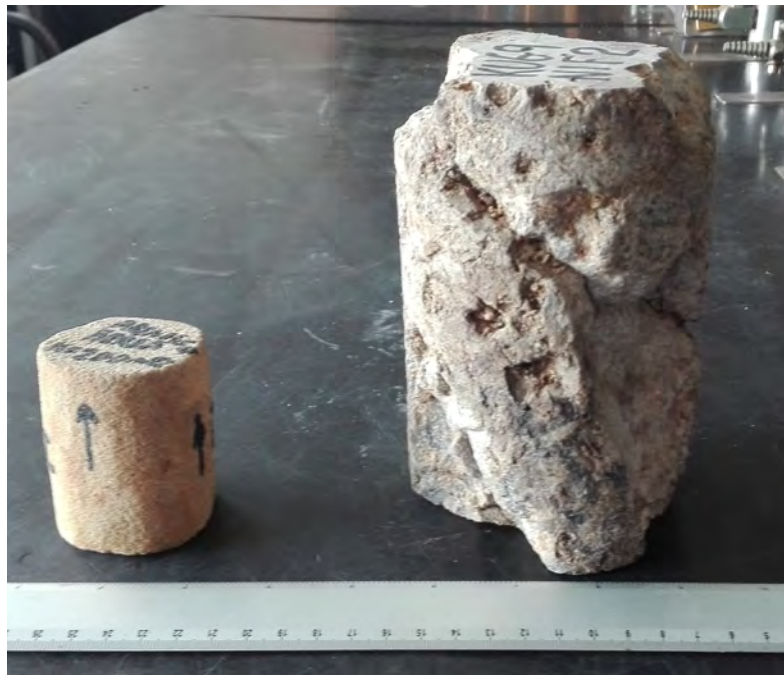
Fig. 1.3: Comparison of plug type samples with whole core samples.
