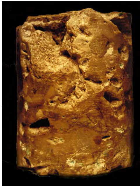
Fig. 2.19: Rock type VII, with representative vuggy- fracture system, with high permeability and porosity in the matrix system.
