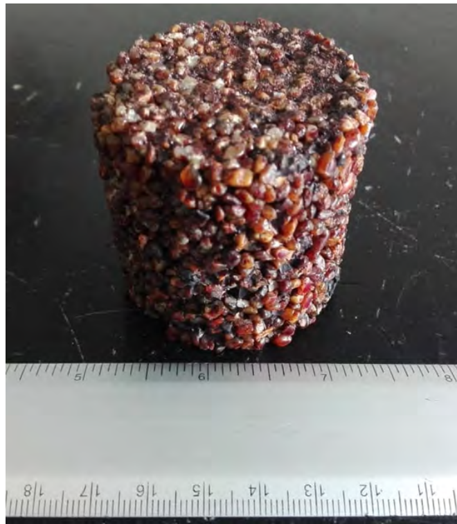
Fig. 2.27: Rock type IX, handmade artificial sandstone rock, homogeneous grain size.
