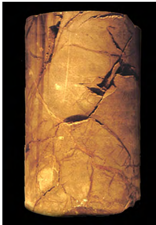
Fig. 2.11: Rock type V, fractured with low matrix porosity and permeability.
