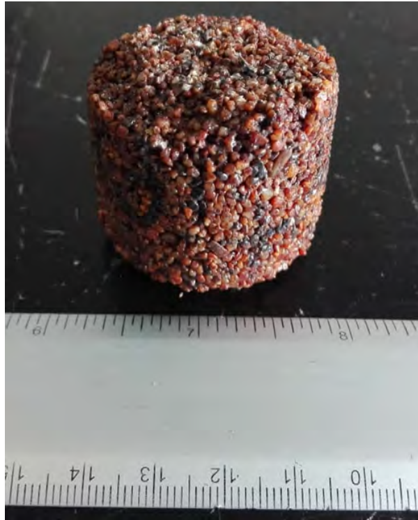
Fig. 2.28: Rock type IX, handmade artificial sandstone rock, variable grain size.
