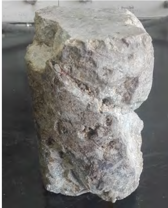
Fig. 2.20: Rock type VII, with representative vuggy- fracture system, with intermediate permeability and porosity in the matrix system. Sample A.
