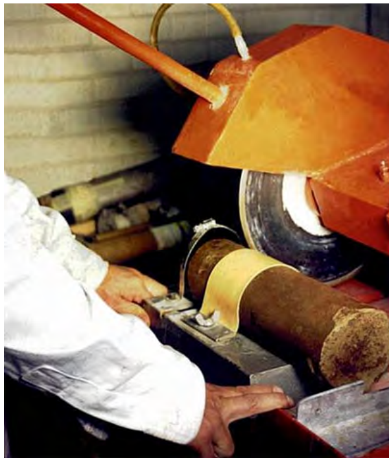
Fig. 4.5: Cut sections of the core selected.
