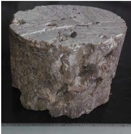
Fig. 2.22: Rock type VII, with representative vuggy- fracture system, with intermediate permeability and porosity in the matrix system. Sample C.
