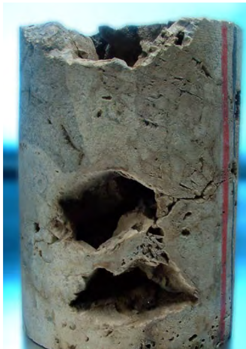
Fig. 2.23: Rock type VII, with representative vuggy- fracture system, with intermediate permeability and porosity in the matrix system. Sample D.
