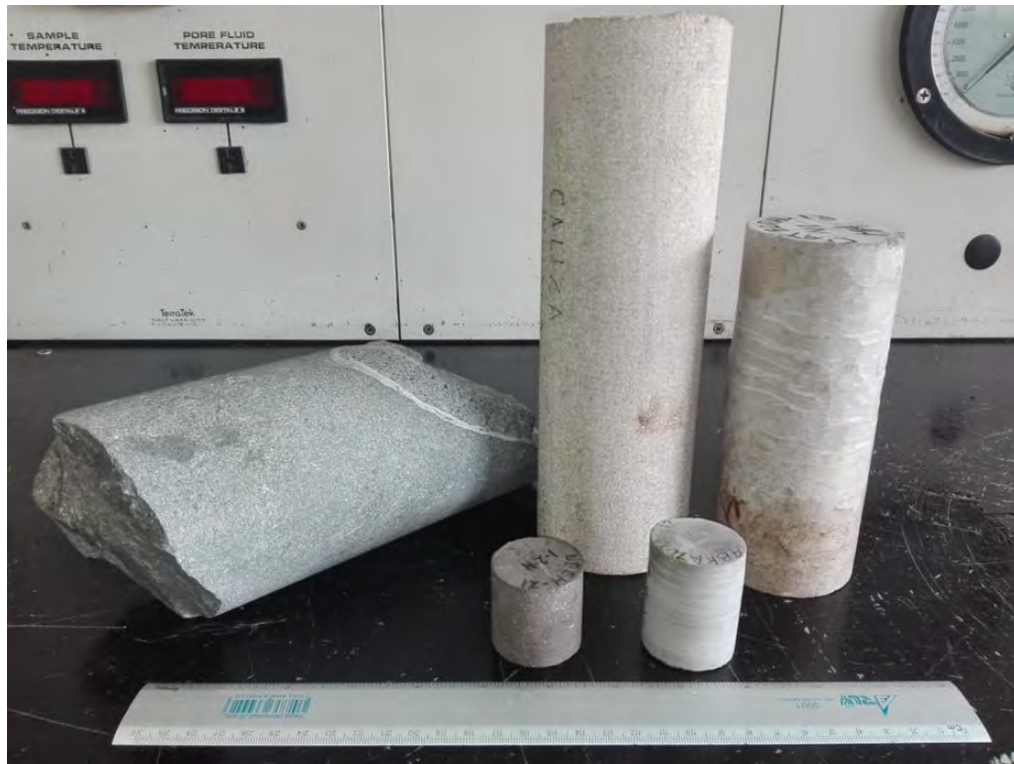
Fig. 2.2: Rock type I, limestone rock samples (very low permeability and porosity matrix).
