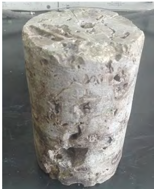
Fig. 2.21: Rock type VII, with representative vuggy- fracture system, with intermediate permeability and porosity in the matrix system. Sample B.
