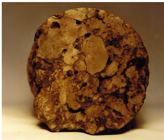
Fig. 2.17: Rock type VII with vugs and intense fracturing.
