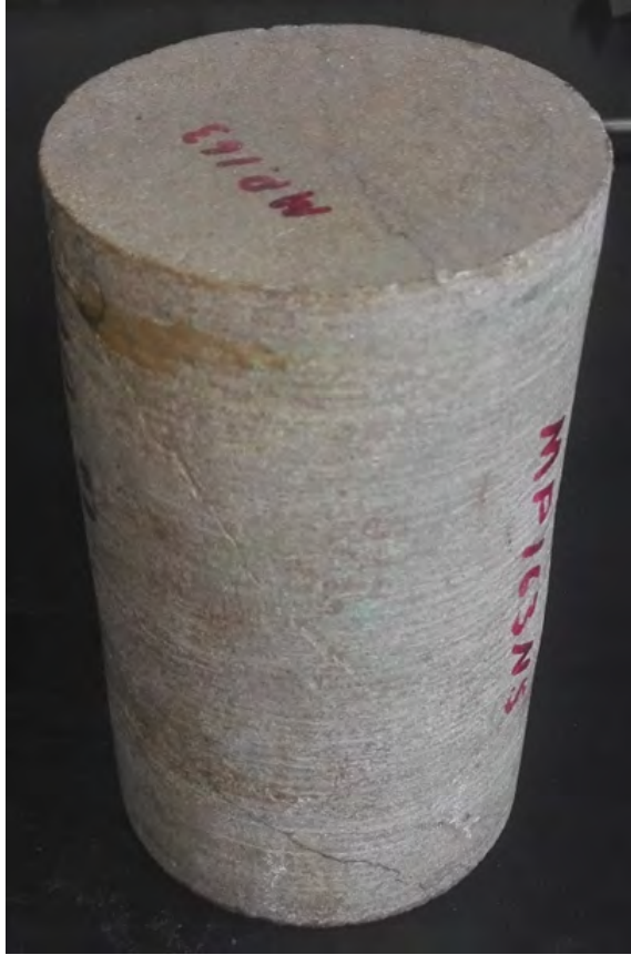
Fig. 2.4: Rock type II, compact full diameter sample 2 (low permeability and porosity).
