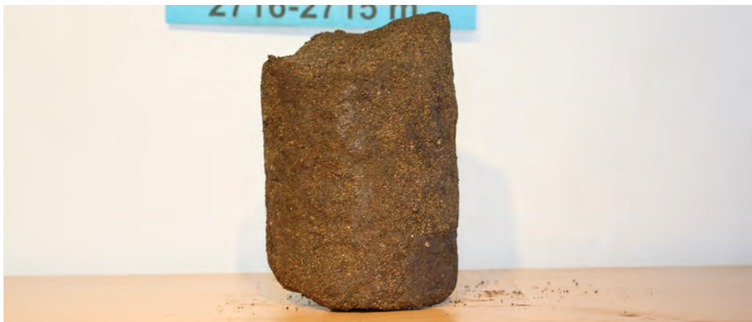
Fig. 2.10: Rock type IV, sandstone of low consolidation. Sample 2.
