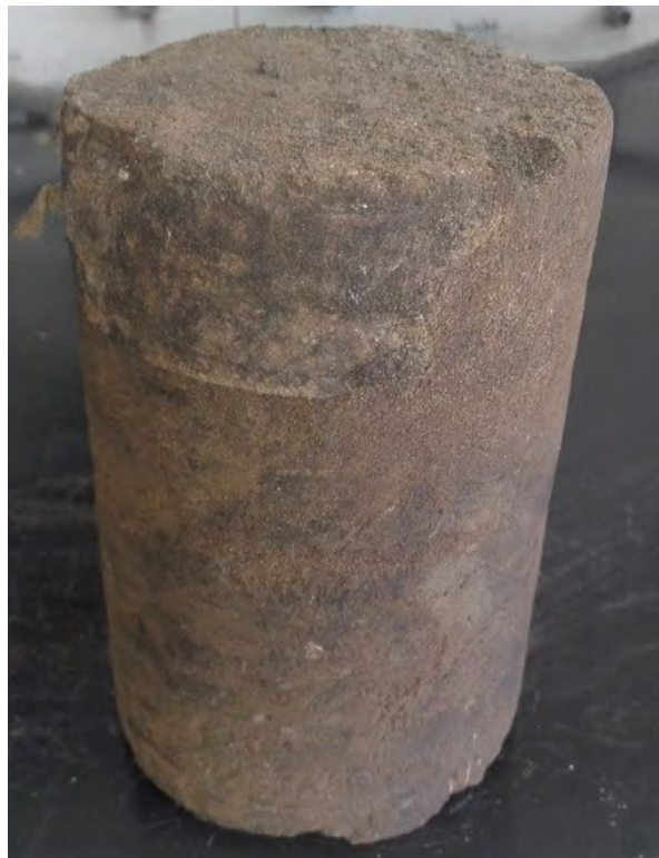
Fig. 2.6: Rock type III, full diameter sandstone 1 with intermediate consolidation.
