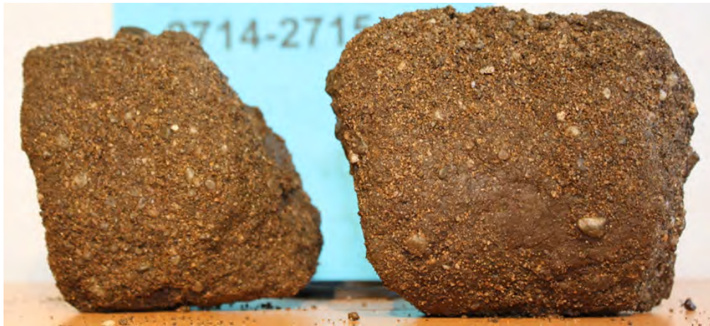
Fig. 2.9: Rock type IV, fragmented rock sandstone of low consolidation. Sample 1.
