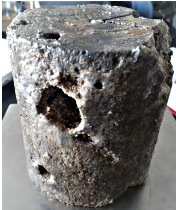
Fig. 1.1: Fractured whole core sample native from naturally fractured oil field from gulf of Mexico.
