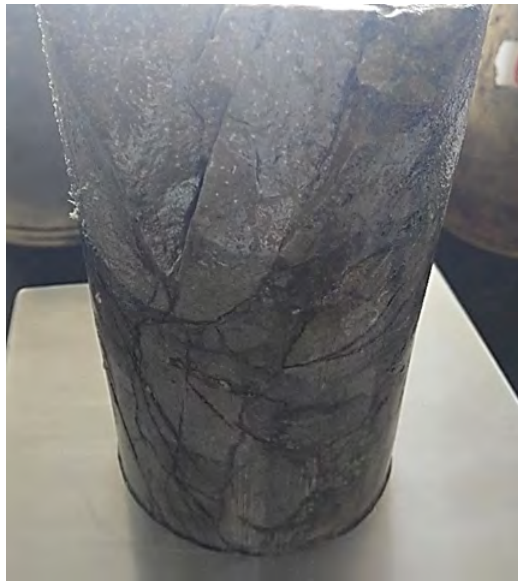
Fig. 2.13: Rock type VI, fractured rock with high porosity and permeability matrix, with irregular and complex geometry.
