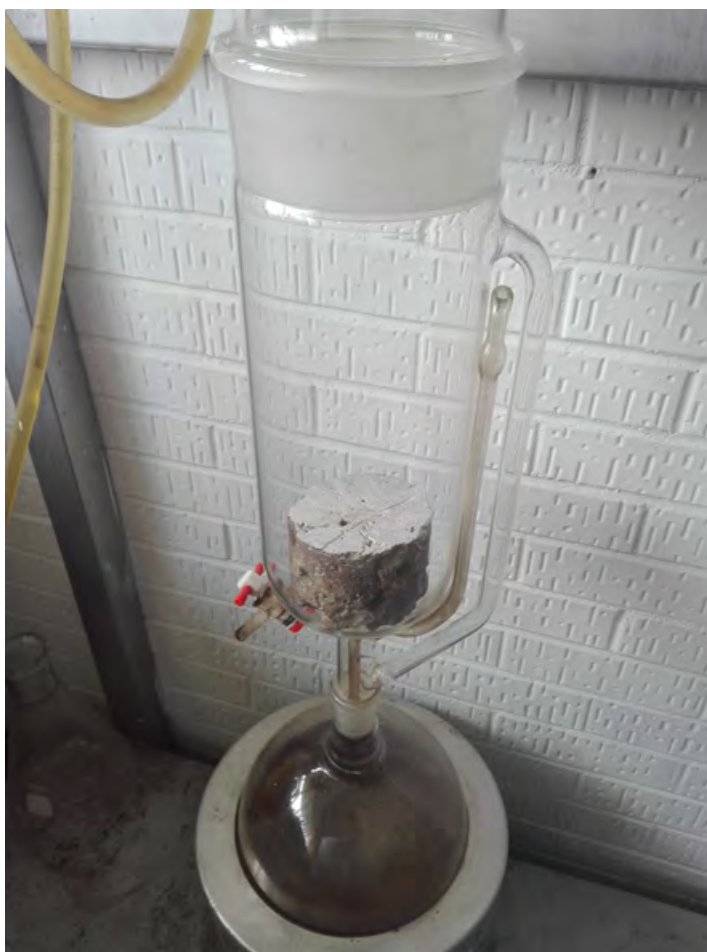
Fig. 4.7: Cleaning of a full diameter sample for an average of 30 days.
