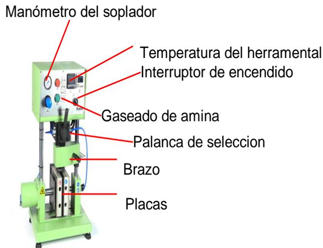
**Figura B.1** Soplador ColdBox (*Simpson test pieces blower*)
