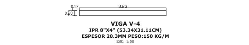
VIGA V-4 IPR 8"X4" (53.34X31.11CM) ESPESOR 20.3MM PESO:150 KG/M ESC: 1:50
