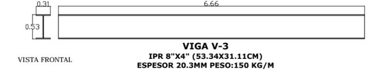
VIGA V-3 IPR 8"X4" (53.34X31.11CM) ESPESOR 20.3MM PESO:150 KG/M ESC: 1:75
