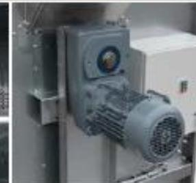
Gear with parallel shaft's makes it easy to turn drum by hand, makes screen change easier.
