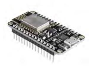
Figura 5.4: Tarjeta NODEMCU<sup>[39]</sup>
