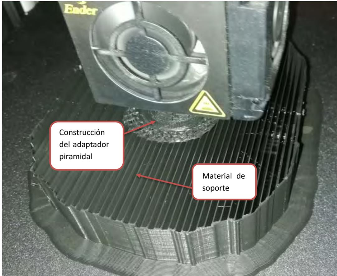
*Fig. 77 Manufactura del socket*
