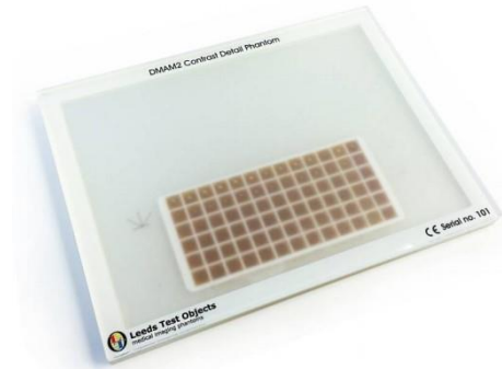
Figura 22: DMAM Gold, de Leeds Test objects
