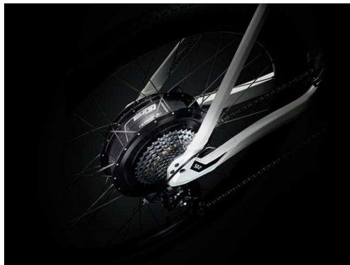
Figura 1.11: Motor tipo geared hub modelo ST2's SYNO Drive Motor [R11].
