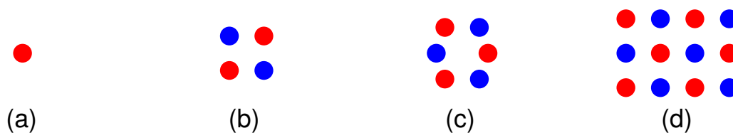
FIGURE 3.3: Geometrical shapes used to arrange the magnets. (a) center, (b) square, (c) hexagon, and (d) checkerboard-magnet arrangement. Blue and red represent north and south poles of the magnet, respectively.
