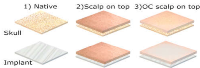
Fig. 2. Stacked sample arrangement used to obtain the spectral transmittance of: 1) the native skull and YSZ implant, 2) the scalp on top of the skull and the YSZ implant, 3) optical cleared (OC) scalp on top of native skull and implant.
