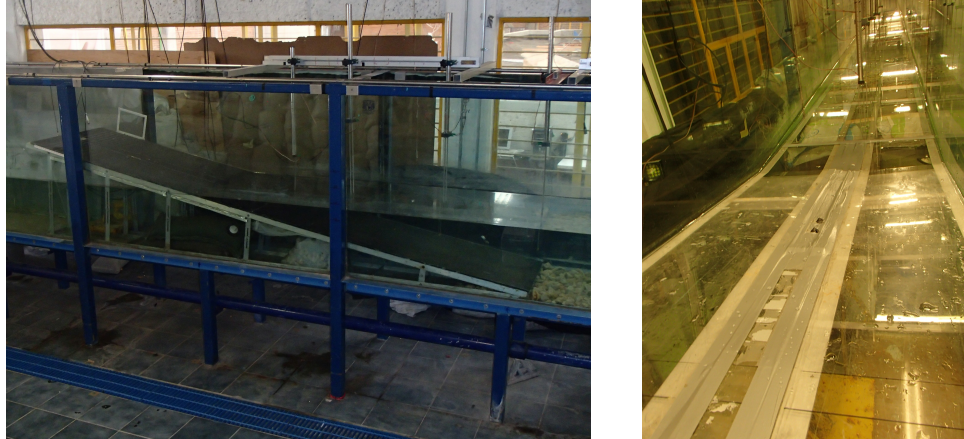
Figure B.2: Ramp metal structure covered with acrylic sheets (right) and with sandpaper (left).
