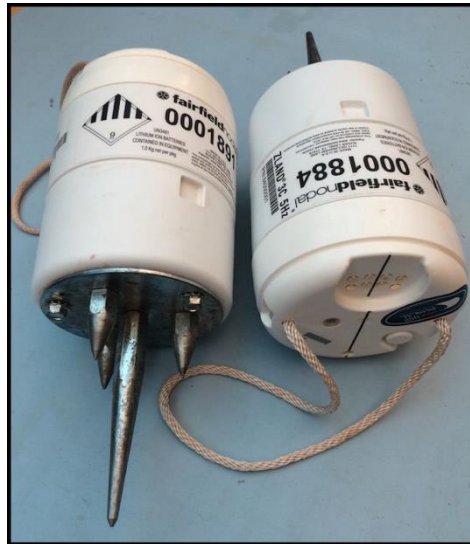
Figura 3.5. Nodos sísmicos Fairfield Z-Land. Tomada de https://www.pascal.nmt.edu/content/fairfielddnodal-zland-3-channel-sensor .
