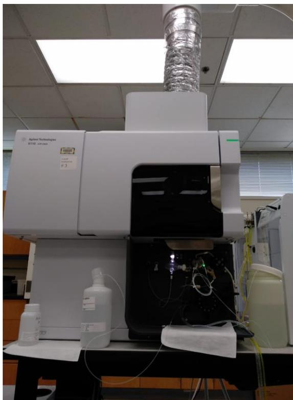
Figura 59. 5110 ICP-EAS Instrument Agilent Technologies
