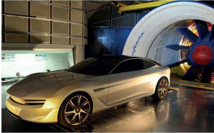
Figure 2.2 Wind tunnel test of an automobile in Pininfarina Cambiano 2012 [53].
