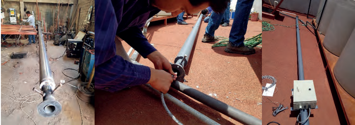
Figure E.6 Process of manufacturing, assembling, and installing the WindMaster anemometer.
