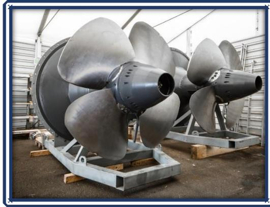
Figura 3.12 - Turbina Kaplan
