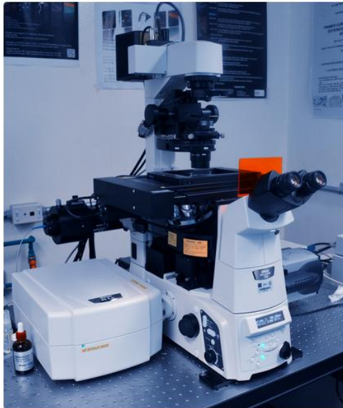
Figura 4.7. Microscopio Confocal Nikon A1R+ STORM [38].
