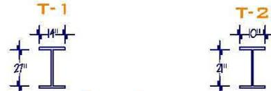
VIGA IPR DE 27" X 14" VIGA IPR DE 21" X 10"
