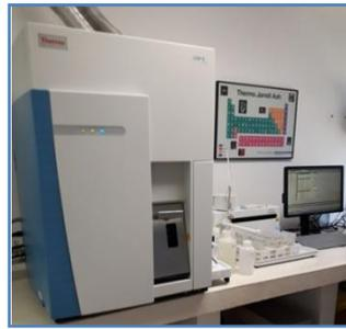
Figura 3.1-7 ICP-MS Thermo Scientific iCap Q.
