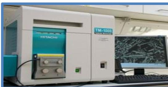
Figura 3.1-4 MEB-EDX Hitachi TM-1000.
