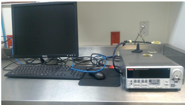
Figura 44. Conductímetro Keithley, 2601B System Source Meter.
