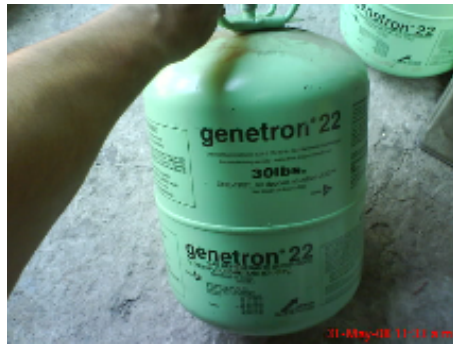
Fig. 2.22 gas refrigerante clorodifluorometano
