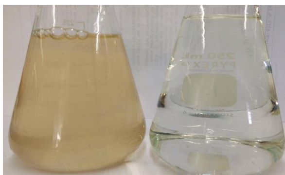
Figure 6. Water treated before (left) and after (right) the microfiltration process.
