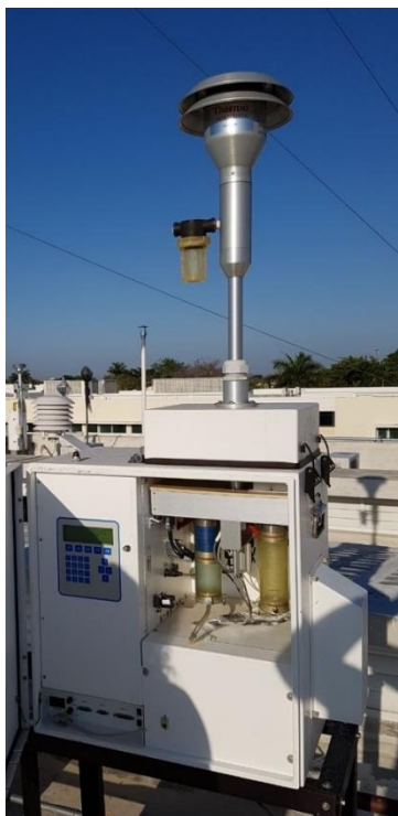
Figura 2.5. Partisol 2025. Thermo Fisher Scientific
