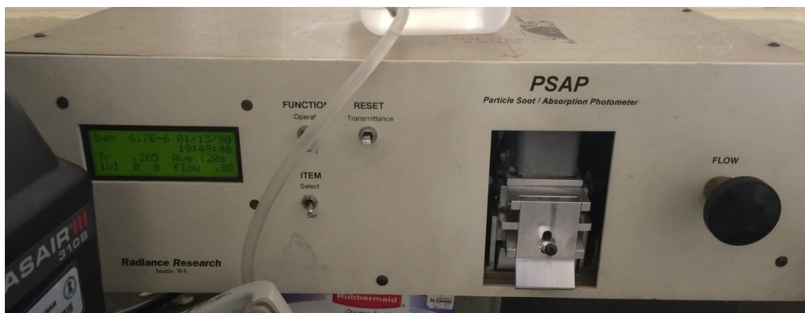
Figura 2.12. Particle Soot Absorption Photometer PSAP, fabricado por Radiance Research.
