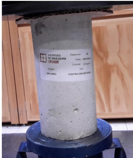
(a) Espécimen de control ensayado (CON, C20-CON, C8-CON).
