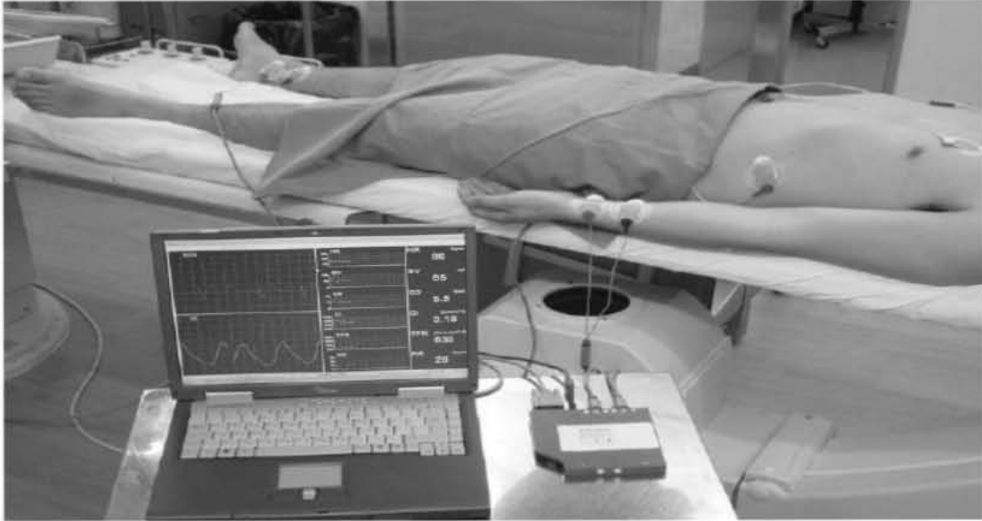
Fig 1. Schema of Non-Invasive Cardiac System, showing the impedance box, which is connected to the patient via proprietary electrodes and the computer that interprets the collected data. Three electrodes are applied to patient's chest for the ECG monitor. One pair of impedance electrodes is applied to the left wrist and another pair to the right ankle (tetra polar mode).
