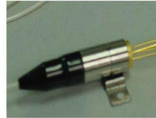
**1310nm or 1550nm DFB Laser - Coaxial Pigtail**
