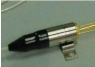
**1310nm or 1550nm FP Laser - Coaxial Pigtail**
