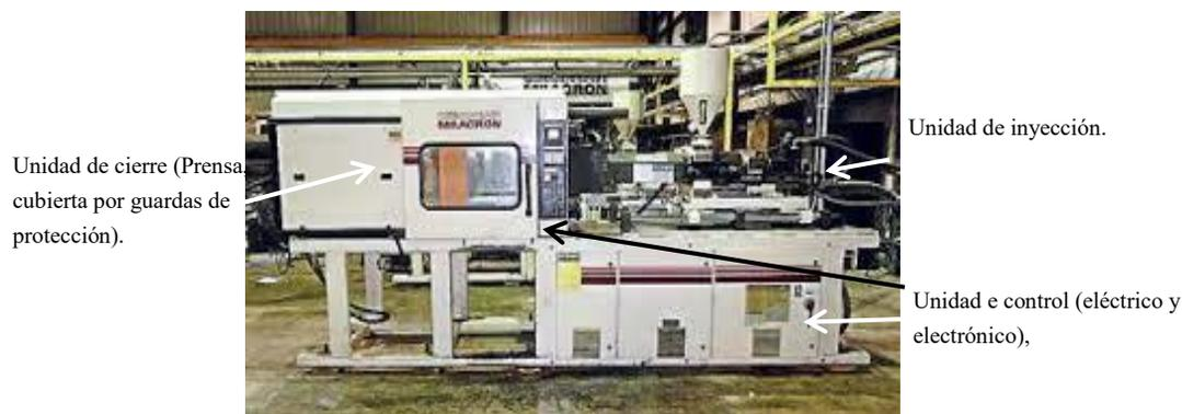
Imagen 3.8. Vista de diversas secciones de una máquina de inyección de plástico. (Imagen tomada de [https://www.stoneauctioneers.com/auctionpages/imm/Stone\\_5.17%20Injection%20Mold%20Auction%20Bro-4.pdf](https://www.stoneauctioneers.com/auctionpages/imm/Stone_5.17%20Injection%20Mold%20Auction%20Bro-4.pdf) para fines educativos).
