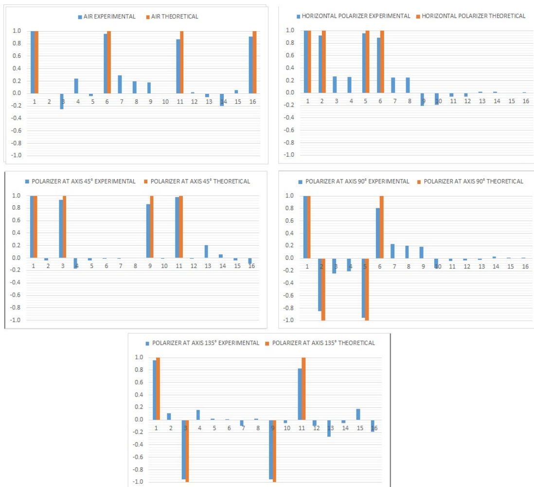
Figure 4.18: Mueller matrices of a known samples, blue lines show the experimental results and the orange lines the theoretical values for air, horizontal polarizer( 0^\circ ), polarizer at 45^\circ , vertical polarizer ( 90^\circ ) and polarizer at 135^\circ , respectively.
