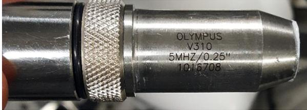
Centrascan Composite Immersion Transducer, 5.00 MHz, 0.25 in. Element Diameter, Standard Case Style, Straight UHF Connector Includes Test Form Certificate.
